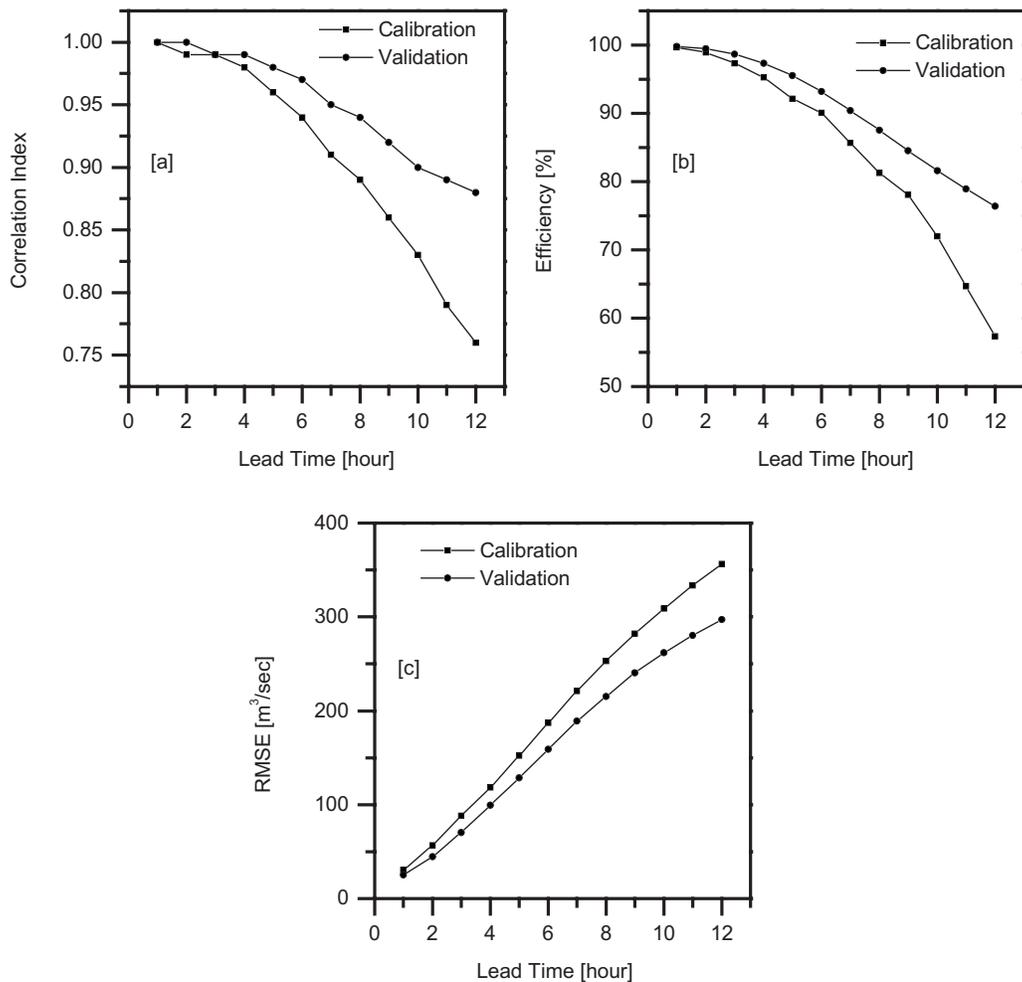
**Fig. 5.** Plot showing different statistical indexes for Model 8 (a) correlation; (b) efficiency; and (c) RMSE
