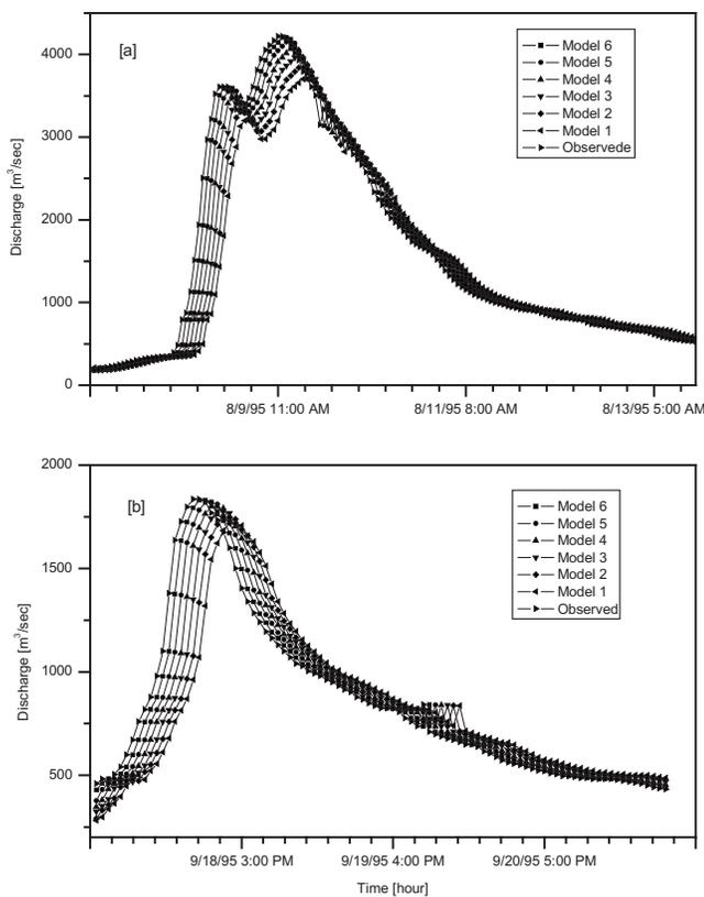
**Fig. 3.** Observed and computed plots for Models 1 to 6 for two flood events
