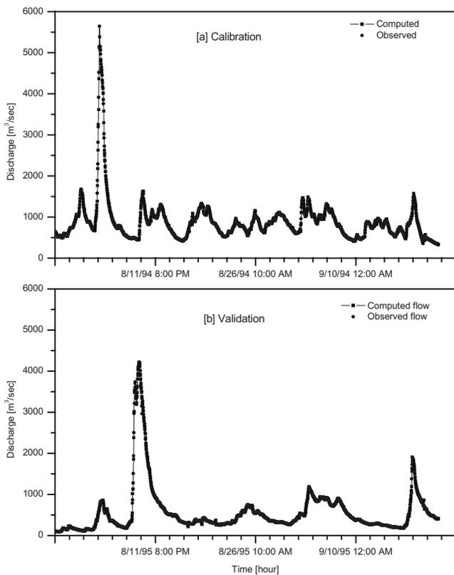
**Fig. 4.** Observed and computed hydrographs for Model 8 for 1-h lead forecast
